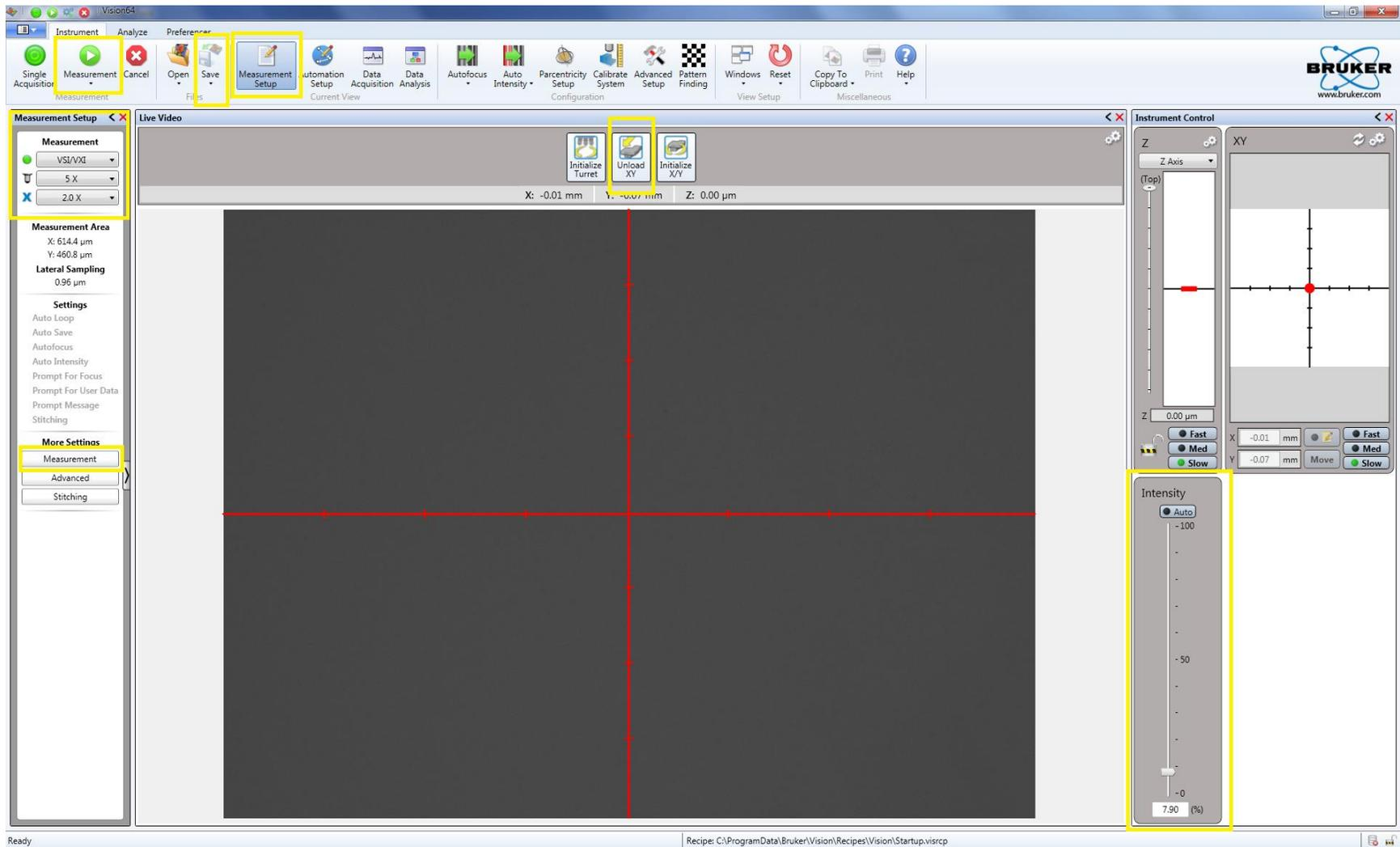
2. Click on **Measurement Setup**. Enter the parameters needed for the sample. Under the **More Settings** option you can access more options for the measurement.
