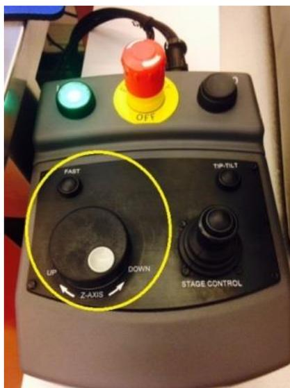
**NOTE: Constantly monitor the gap between the objective lens and sample while adjusting the Z position. Crushing the objective lens to sample will seriously damage the instrument and result in expensive repair.**
