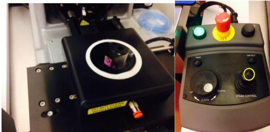
4. Focus on the surface by moving the stage up using the **“Z-Axis”** control. (Pressing the **“Fast”** button moves the stage faster)
