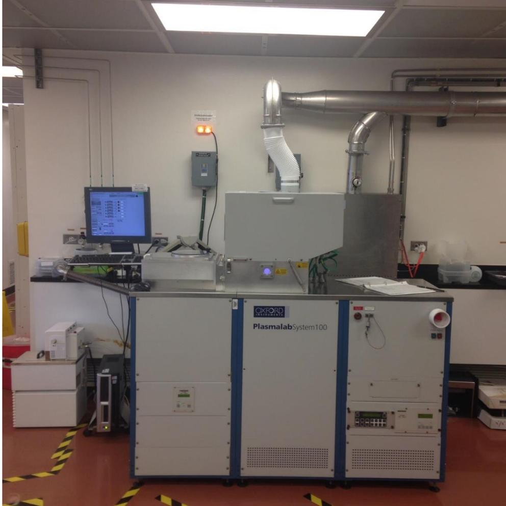
The Oxford Deep Reactive Ion Etching system is used for highly anisotropic etch processes, creating deep penetration, steep-sided holes and trenches in wafers/substrates with high aspect ratios. The main process used on the NCF system is the Bosch etching process, although other process can be programmed. The Bosch process can fabricate 90° walls, but often the walls are slightly tapered, e.g. 88° ("reentrant") or 92° ("retrograde").
