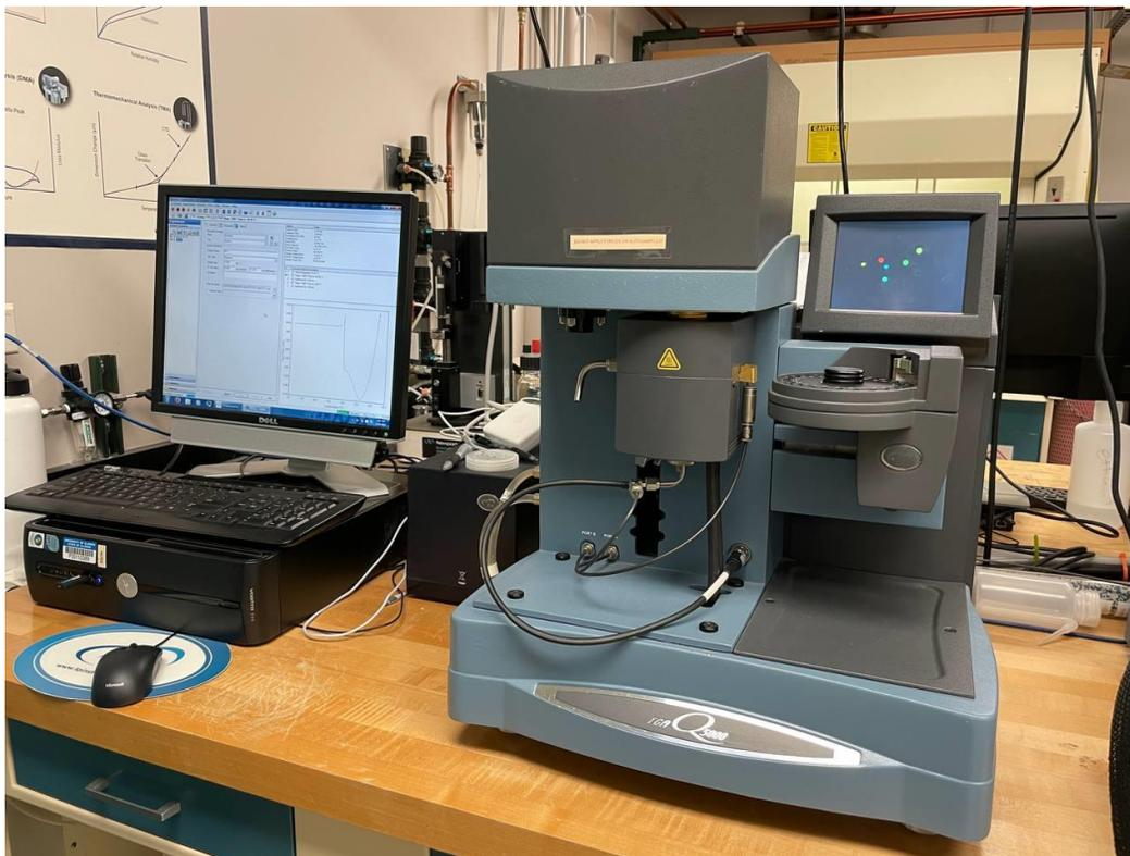
Thermogravimetric analysis (TGA) is a weight change analysis system. The Thermogravimetric Analyzer measures the amount and rate of weight change in a material, either as a function of increasing temperature or isothermally as a function of time, in a controlled atmosphere. It can be used to characterize any material that exhibits a weight change and to detect phase changes due to decomposition, oxidation, or dehydration.
