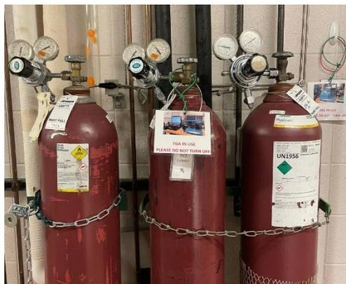
2. Open the gas valve by the wall next to the instrument.
