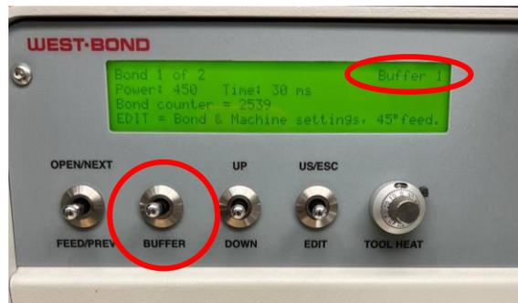
Each of the buffers holds the bond settings and bonds per wire data. By assigning a buffer number for your sample, you won't need to set up the parameters again in your next usage.
